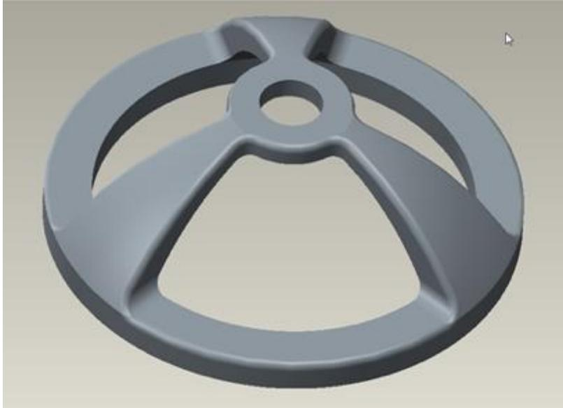
Figure 6: 3D view of the dome structure to be printed at the Head to Head Competition
